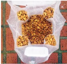
The unique EcoCube™ bag features five chambers. The CVC BT Vibratory Belt Table ensures that ingredients are level in all chambers before closing and sealing.
